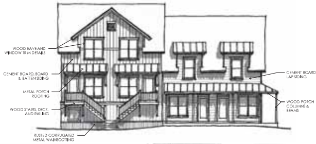
Building Type C Street Elevation
