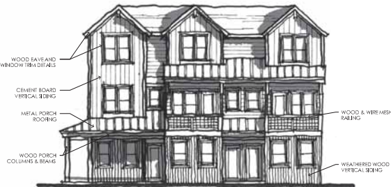
Building Type E Street Elevation
