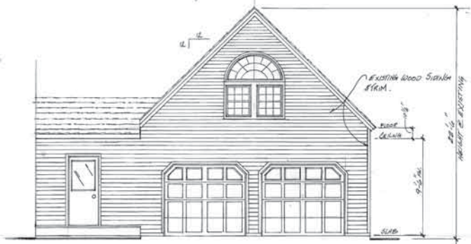
FRONT ELEVATION OF GARAGE 1/4" SCALE (EXISTING CONDITIONS)
