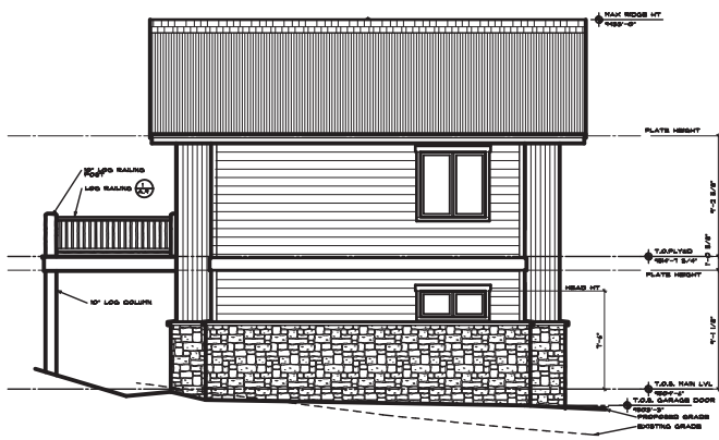
3 NORTH EAST ELEVATION A-E
