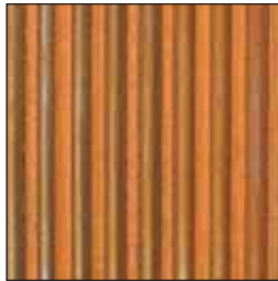
METAL ROOFING: COLD ROLLED STEEL (RUSTING)
