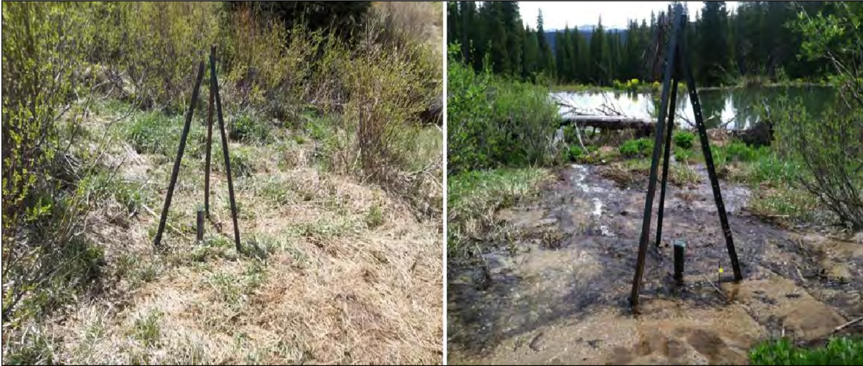
Photo C5. Deposition at Well A. The left photo shows Well A in 2012 and the right photo shows it during runoff in 2014 (from a different angle). The flowing water is outflow from the lateral spreader ditch. Note the amount of sediment deposition.
