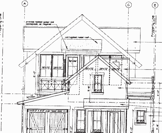
1 East Elevation Scale: 1/4" = 1'-0"
