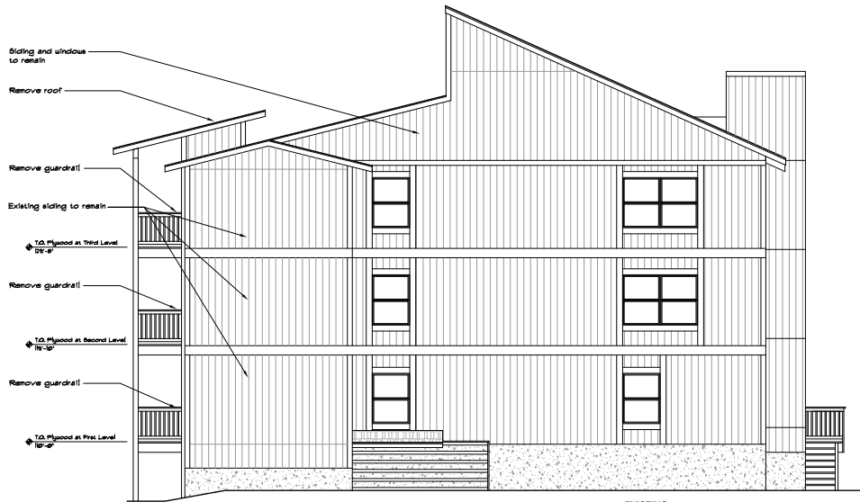
EXISTING NORTH ELEVATION 3/16"=1'-0"
