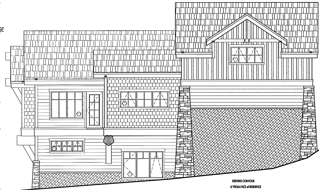
BUILDING 'H' - WEST ELEVATION SCALE : 1/4" = 1'-0"
