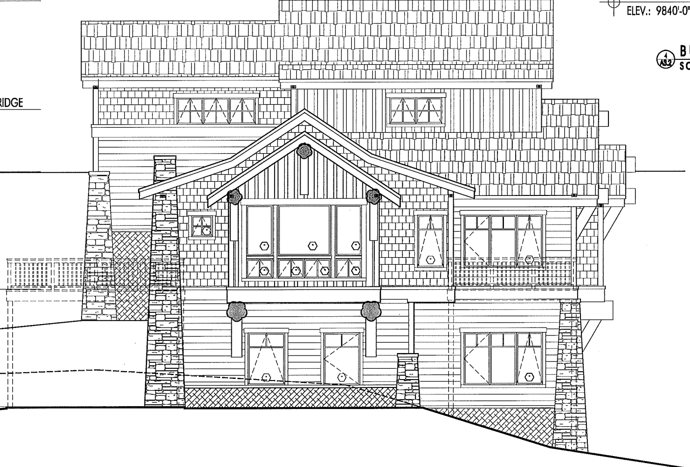
BUILDING 'F' - NORTH ELEVATION SCALE : 1/4" = 1'-0"
