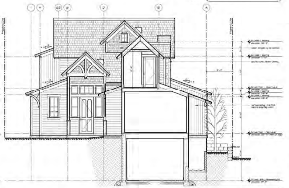
2 A-7 West Building Section Scale: 1/4" = 1'-0"
