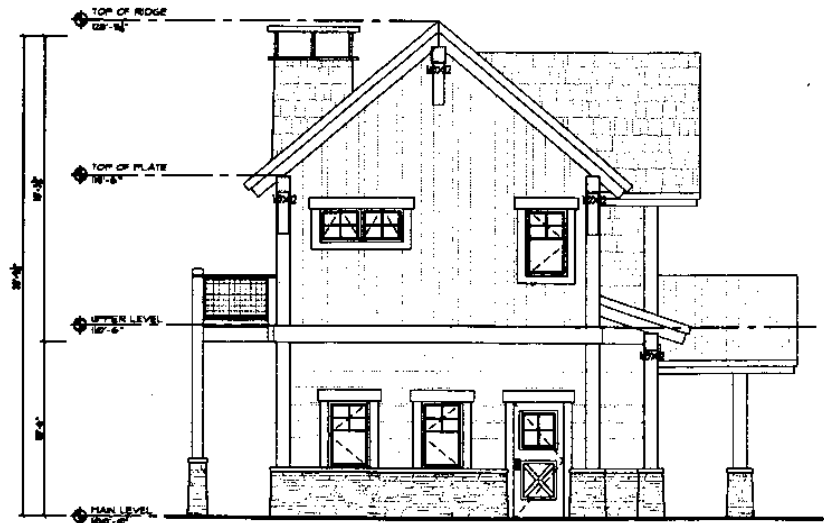
4 EHU BUILDING - SIDE ELEVATION AEHU 5.1/4" = 1'-0"
