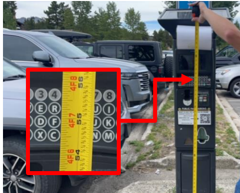
Measurement of operable part is too high. 48" maximum.
