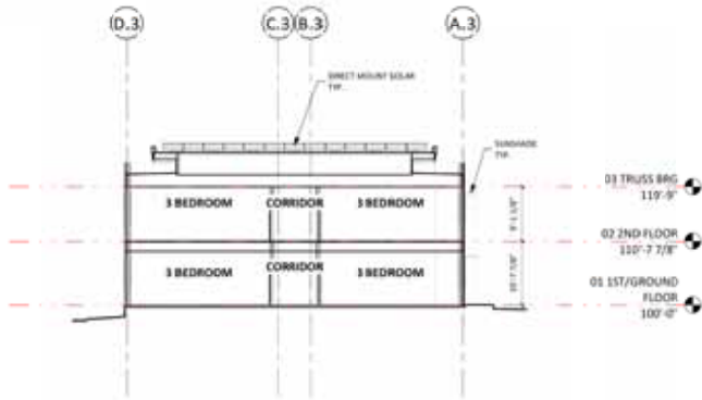
2 BUILDING 3 SECTION - TRANSVERSE 1 SCALE: 3/16" = 1'-0"
