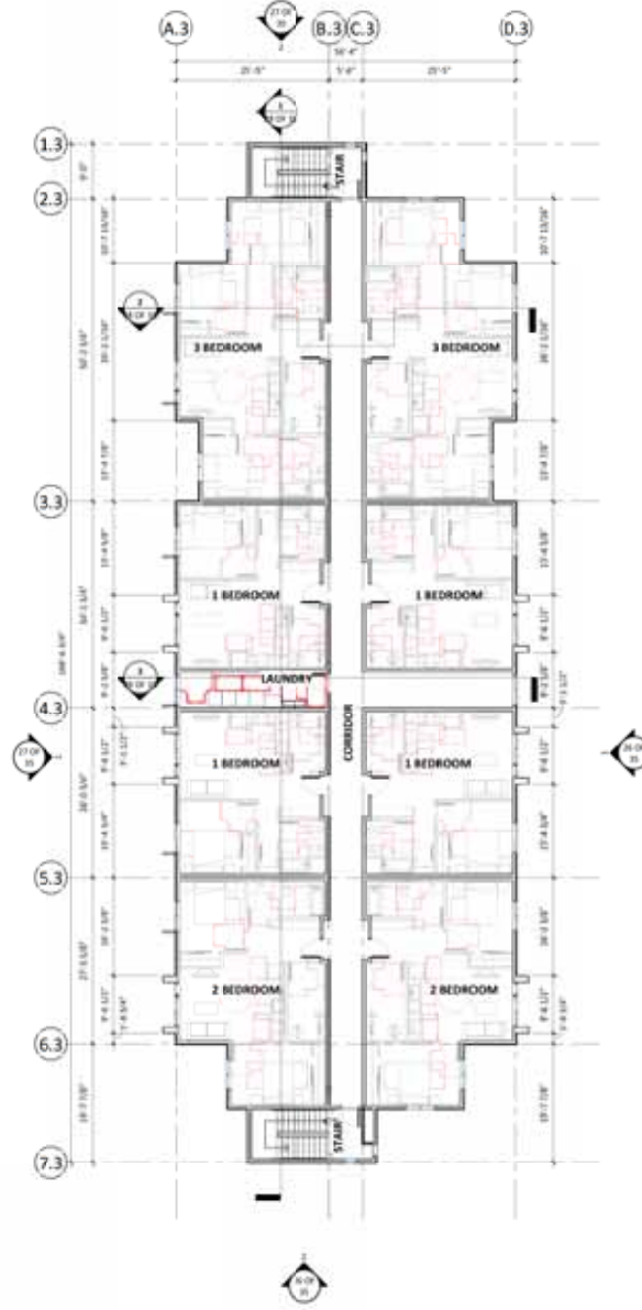
2 BUILDING 3 SECOND FLOOR SCALE: 1/32" = 1'-0"
