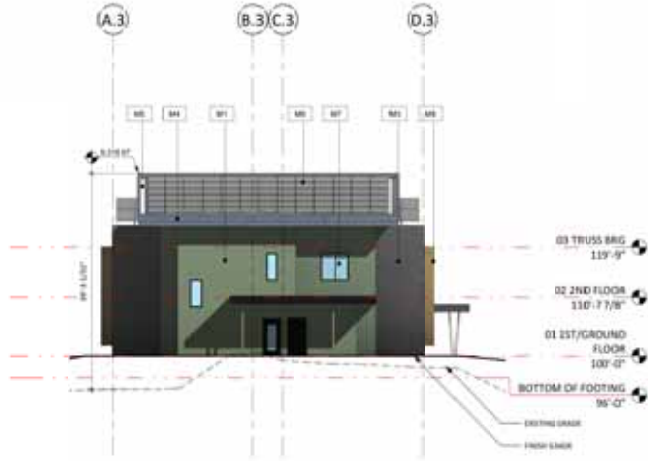
2 BUILDING 3 - SOUTH ELEVATION SCALE: 3/32" = 1'-0"
