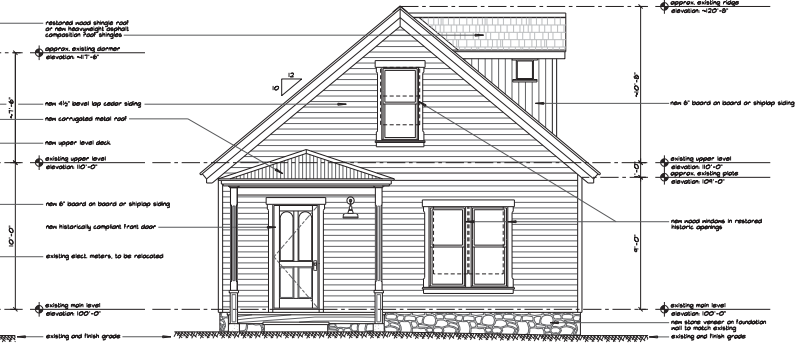
West Elevation Scale: 1/4" = 1'-0"
