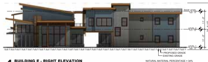
4 BUILDING E - RIGHT ELEVATION 3/32" = 1'-0"
