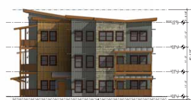
2 BUILDING C - RIGHT ELEVATION
