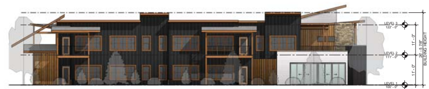
1 BUILDING E - FRONT ELEVATION 3/32" = 1'-0"
