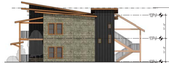
4 BUILDING A - RIGHT ELEVATION 1/8" = 1'-0"
