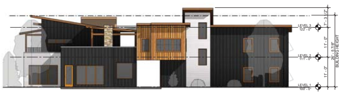
4 BUILDING E - RIGHT ELEVATION 3/32" = 1'-0"
