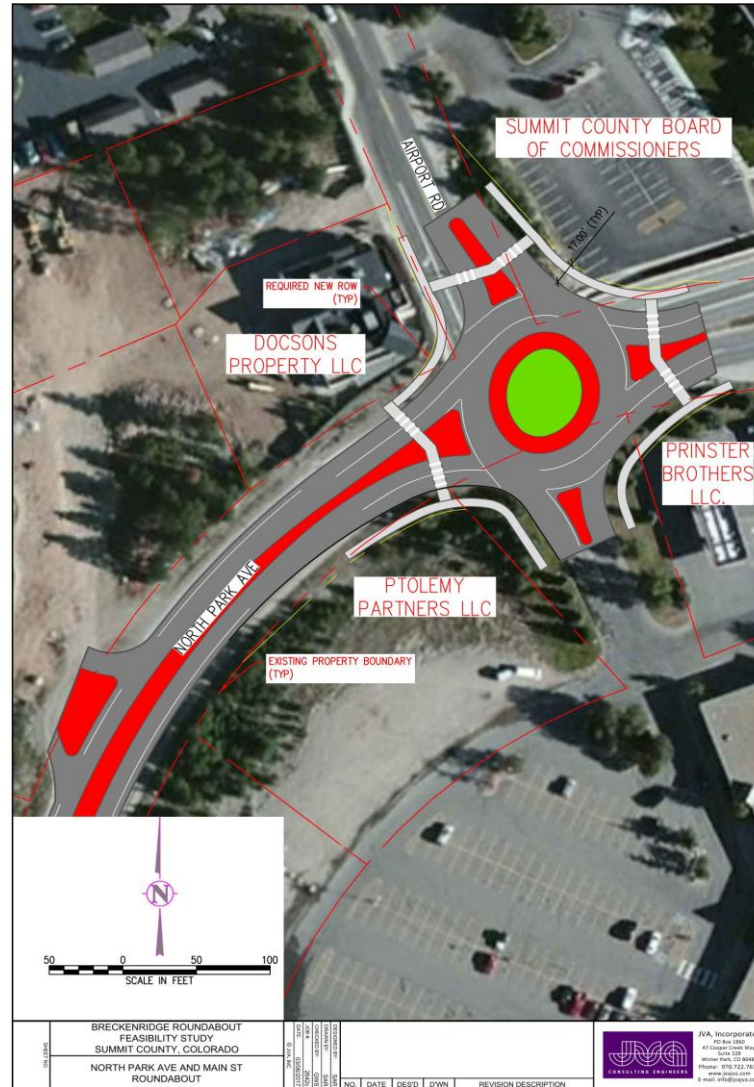
Conceptual Roundabout Layout at Airport Road & Park Ave
