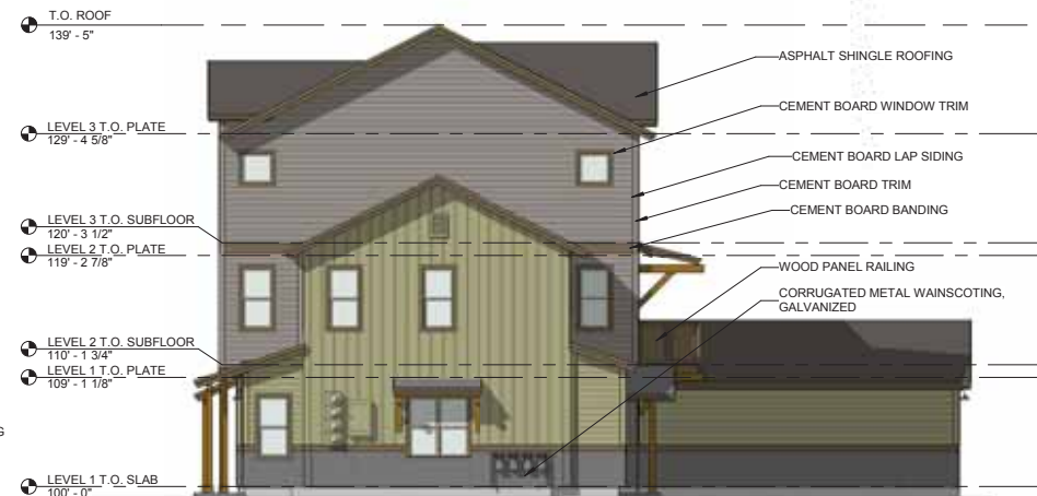
1 RIGHT ELEVATION (INTERNAL OR STREET) 1/8" = 1'-0"
