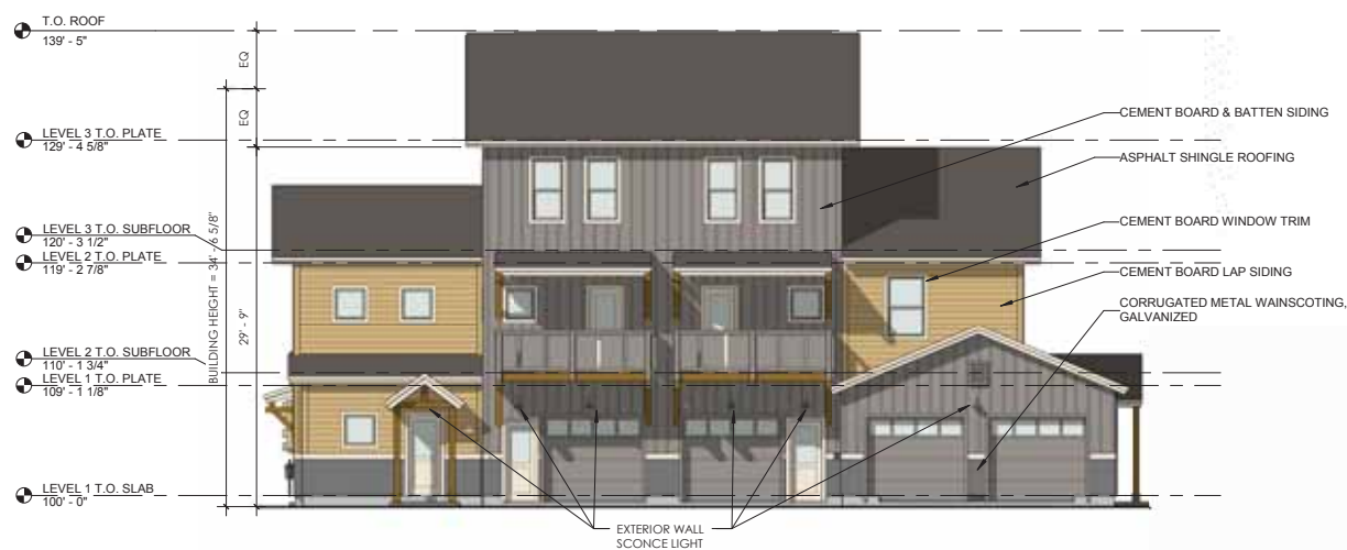
2 BACK ELEVATION (ALLEY) 1/8" = 1'-0"
