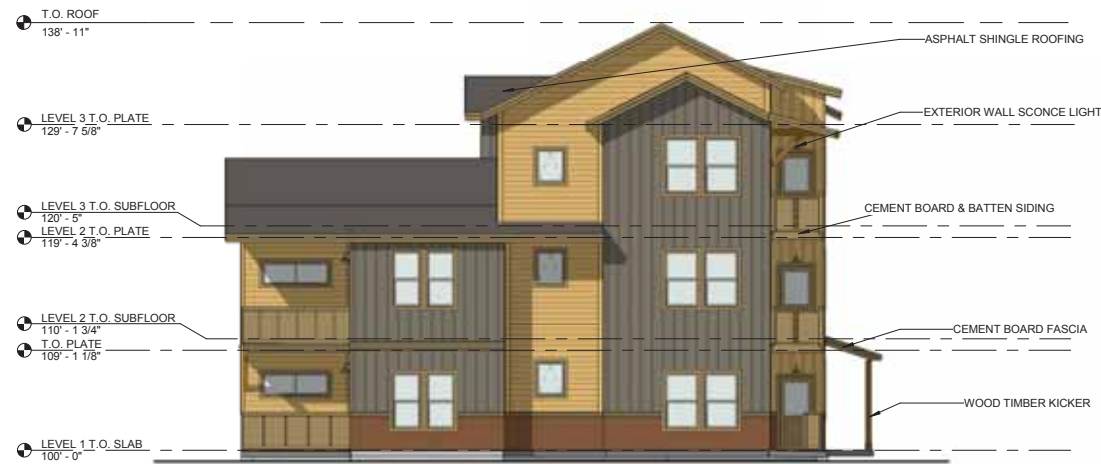
4 Left Elevation (Internal) 1/8" = 1'-0"
