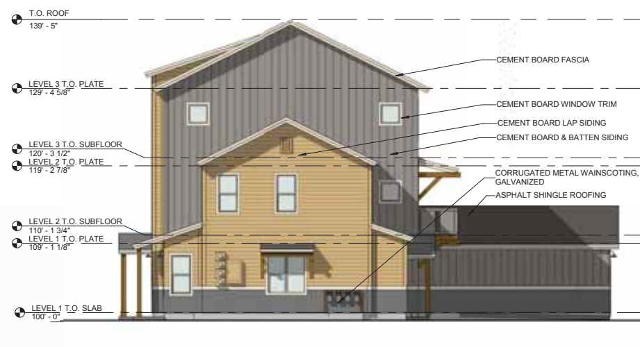
1 RIGHT ELEVATION (INTERNAL OR STREET) 1/8" = 1'-0"
