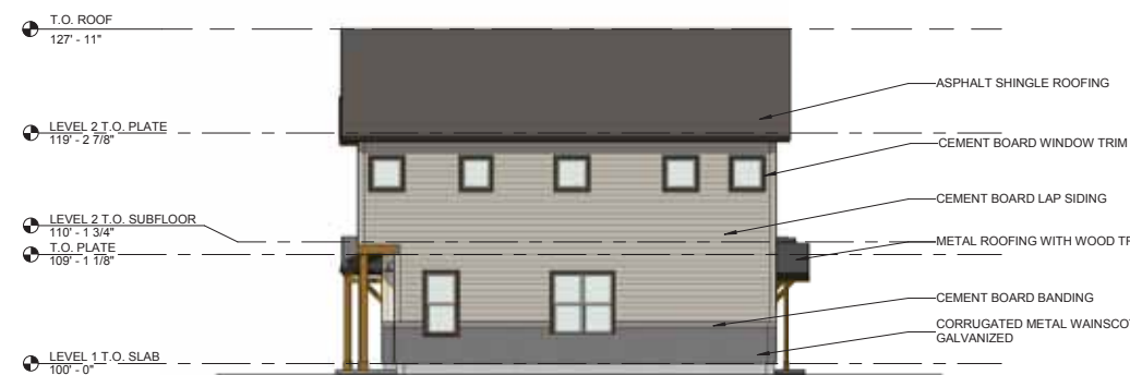
3 Right Elevation (Internal) 1/8" = 1'-0"
