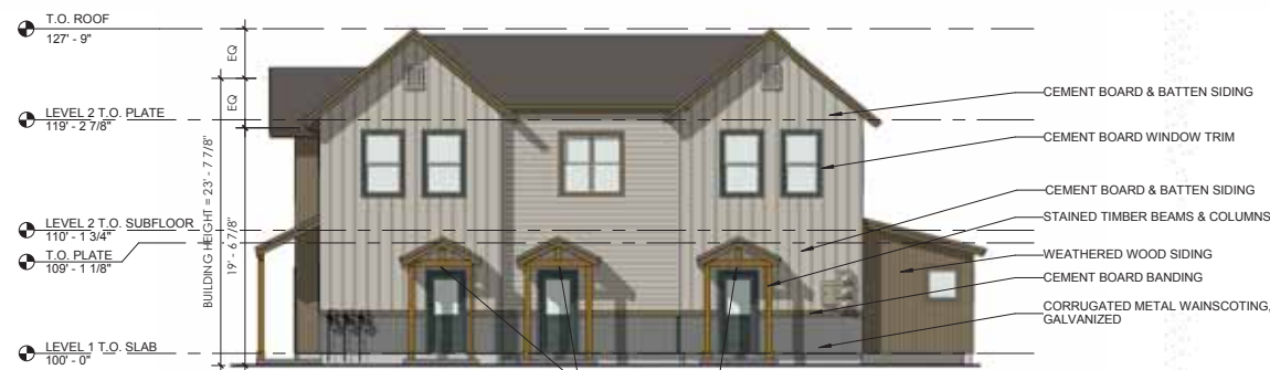
2 Back Elevation (Parking) 1/8" = 1'-0"
