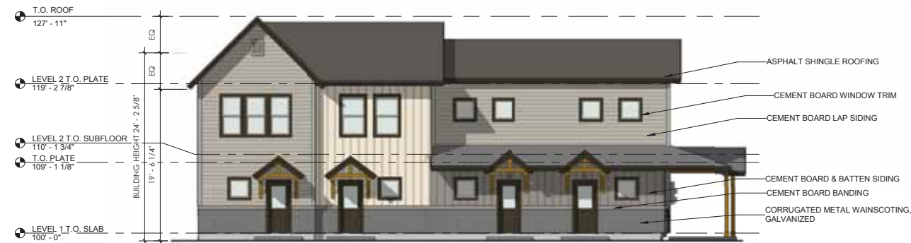
2 Back Elevation (Internal, CMC) 1/8" = 1'-0"
