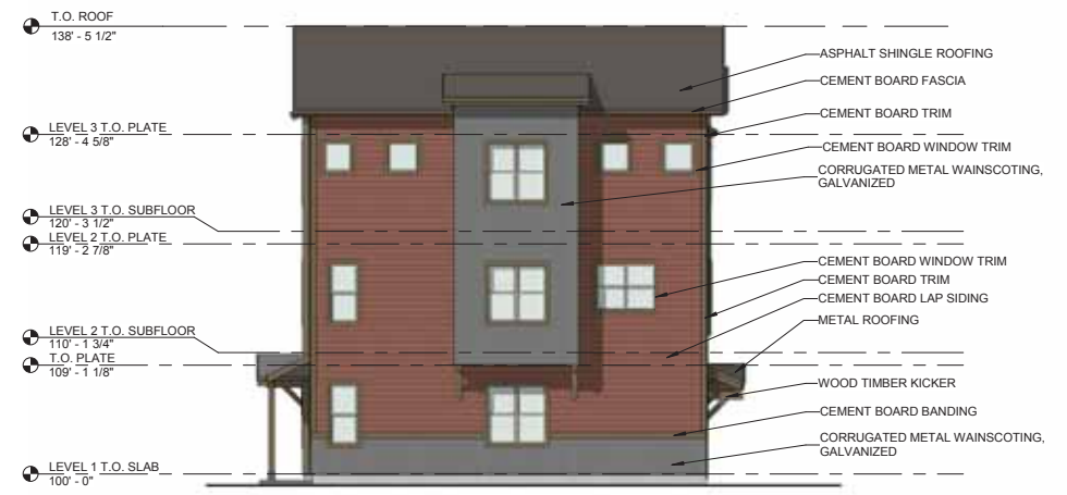
5 Right Elevation (Internal) 1/8" = 1'-0"
