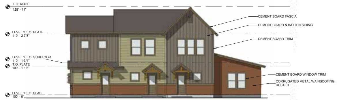
2 Back Elevation (Internal, CMC) 1/8" = 1'-0"
