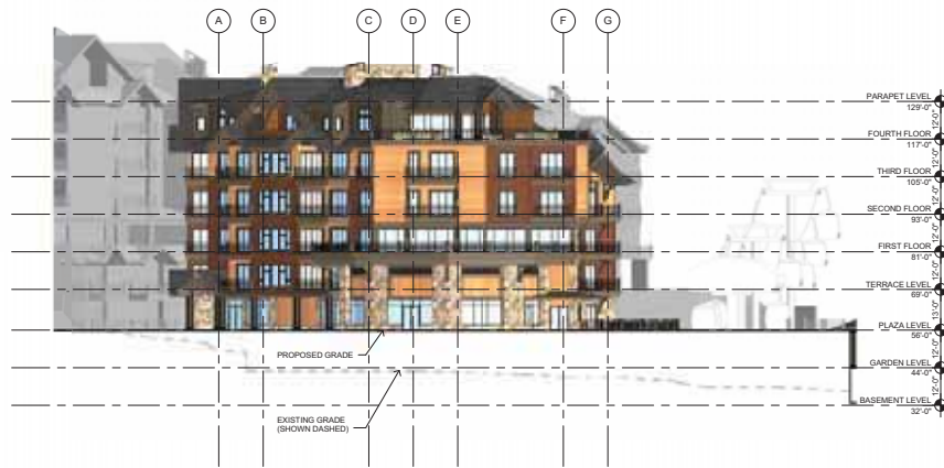
2 A301 COMPOSITE SOUTH ELEVATION SCALE: 1/8"=1'-0"
