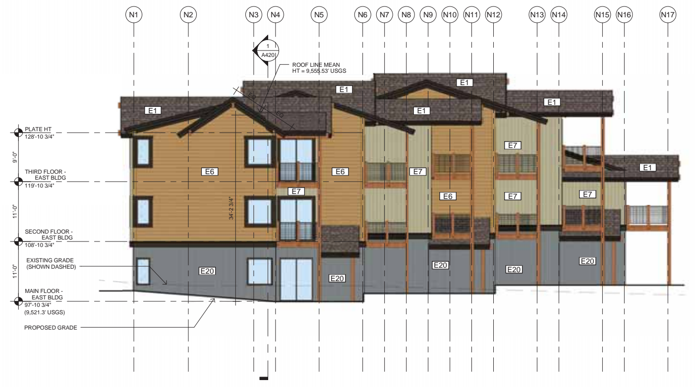
2 WEST ELEVATION - EAST BLDG A320 SCALE: 1/8" = 1'-0"
